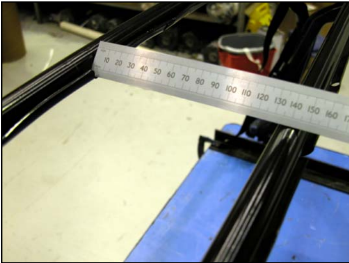
Picture 3. Check straps provide a gap of 130mm between the 2nd and 3rd (rear) frame bows.
