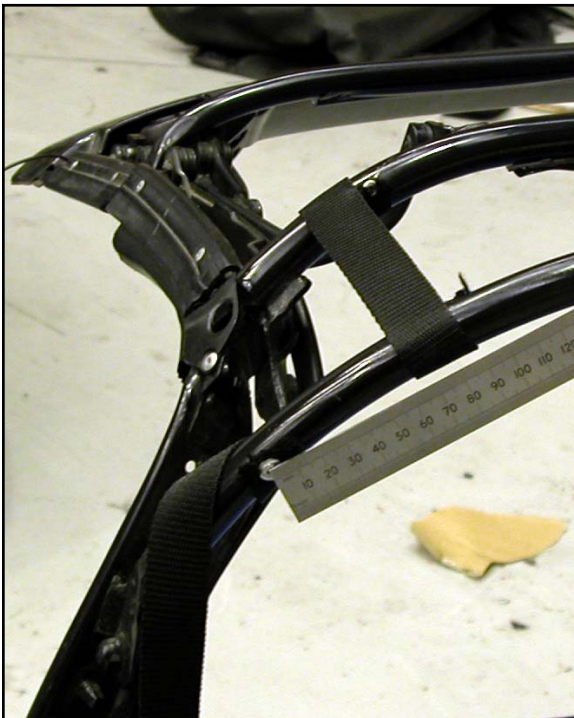
Picture 5. Long strap is riveted to rear frame bow as shown 70mm from short strap location.
