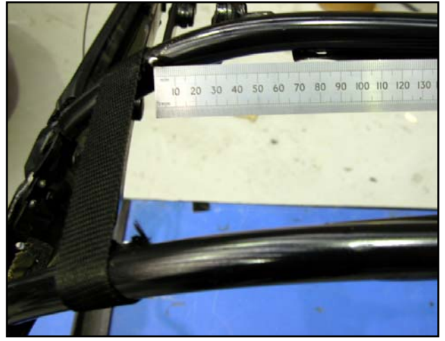
Picture 2. The straps are positioned 70mm from the frame slots.
