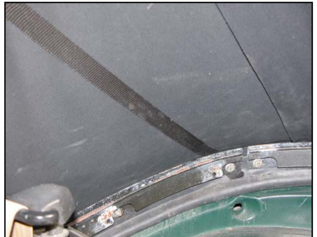
Picture 6. Long strap locates behind rear retaining bar during installation of the hood to the car.
