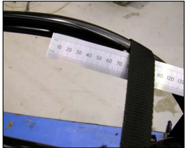
Picture 4. Short strap wraps over top of frame bow and back under. Rivet as shown 70mm from frame slot.
