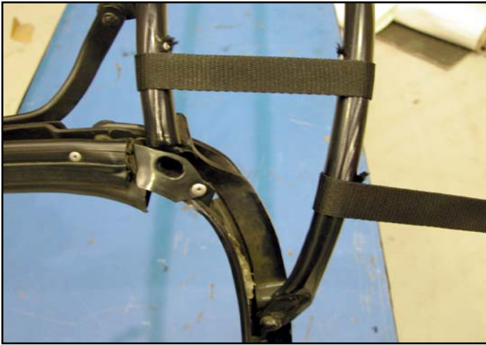
Picture 1. The frame straps are riveted to the 2nd and 3rd (rear) frame bows.
